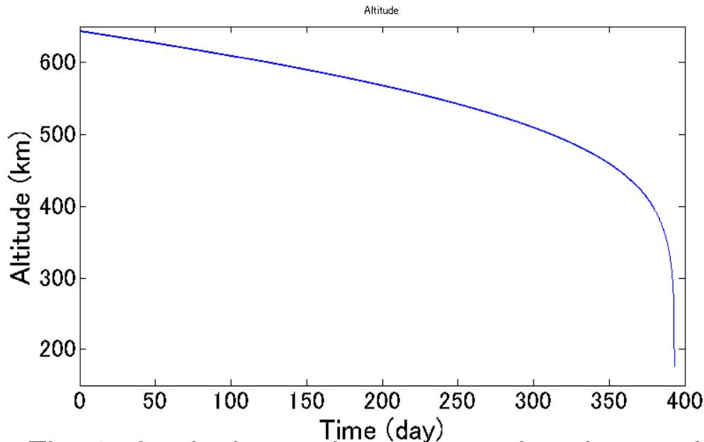
Fig. 2. Analysis results representing descend trajectories using the proposed de-orbit system.
